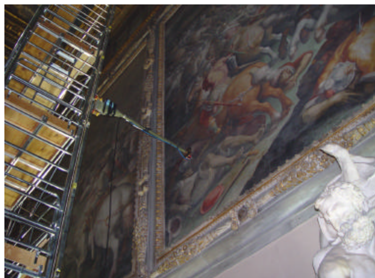
Figure 2: Radar inspection of a painting by Vasari, Sala del 500, Firenze, Italy.
